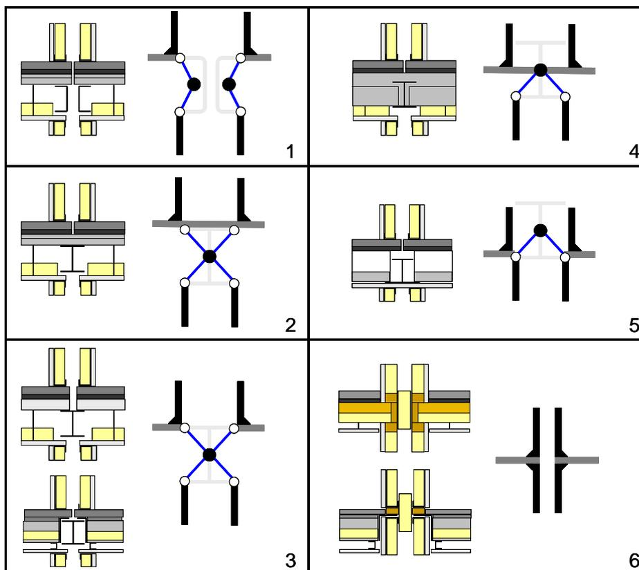
Figure 1: The required six types of boundary conditions to model all relevant types of lightweight junctions.
