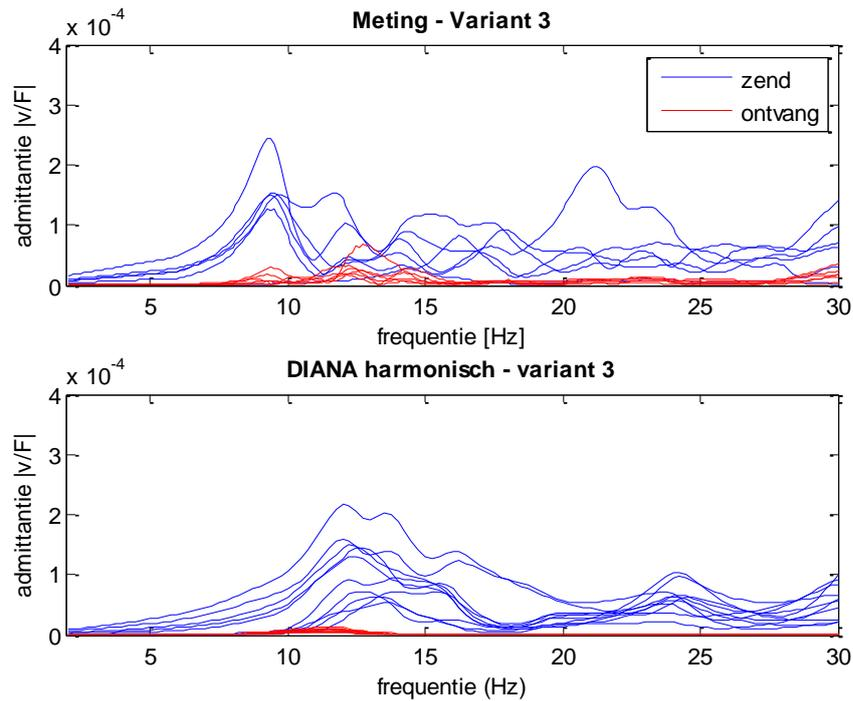
Figure .3: Comparison between the measured and the predicted transfer mobility of the junction without floor screed (meting=measurement, DIANA harmonisch=prediction, admittantie = mobility= transfer function, zend = send, ontvang = receive, frequentie=frequency)
